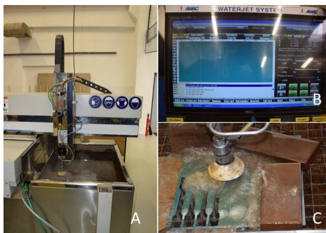
Fig. 1. Machining of polymeric composites by means of water-jet technology: A: CNC AWJ CT 0806, B: Water-jet system, C: Production of test samples, composite board cutting
